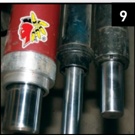
▲ LARGE 4" CYLINDERS equal longer seal life and lower operating pressures vs. smaller competitive cylinders.
