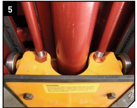
▲ Each carriage rolls on (8) 4" double sealed, self lubricating, heavy duty ball bearing rollers for a lifetime of trouble-free service (not plastic slide blocks).
